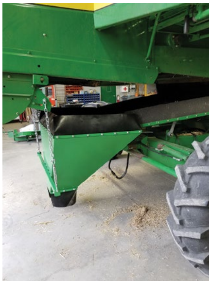
↑ AAFC had this chaff lining chute built specifically for this project. It cost about $5,000. Credit: Louis Molnar
