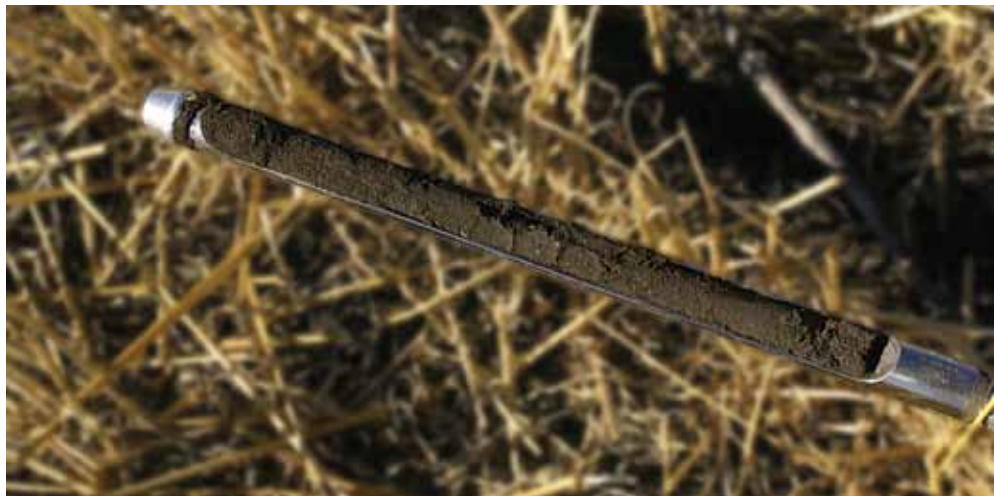
Soils can still be sampled during the winter, as long as the probe can still get down 24".
