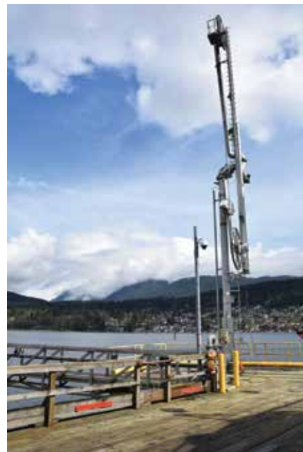
Pacific Coast Terminal in Port Moody, B.C., built a facility to handle canola oil, with train unloading (shown on the cover with PCT’s Clayton Smith), 45,000 tonnes of storage tank capacity and a ship-loading pump (shown above) that can move 1,100 tonnes of oil per hour.
